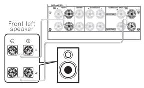
Since both front and surround back speaker terminals output the same audio, it doesn't matter which set (front or surround back) is powering which part (**Hi** or **Low**) of the speaker.
